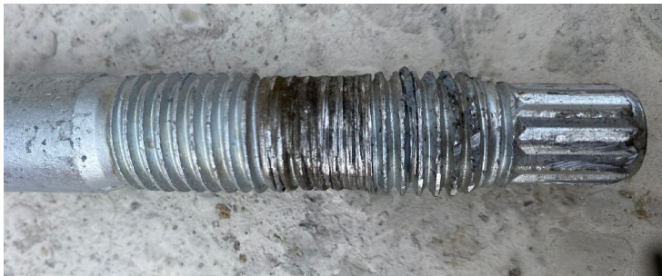
Example 1: Thread Stripping
