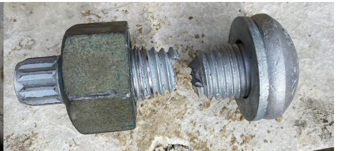
Example 2: Torsional fracture
