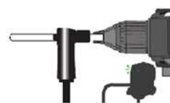
Hollow drill bit (Dustless drilling)
